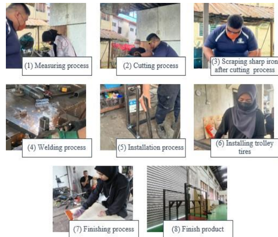
Pictures (1-8): showed the trolley fabrication process.
